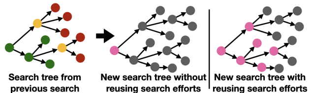
Fig. 3: Visualization of how we reuse search efforts. Reusable nodes are in green, boundary nodes are in yellow and non-reusable nodes are in red. Pink nodes are obtained directly from previous search while gray nodes are newly constructed in the current search.
